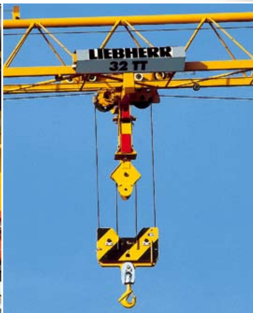
Patented automatic rope re-reeving.
