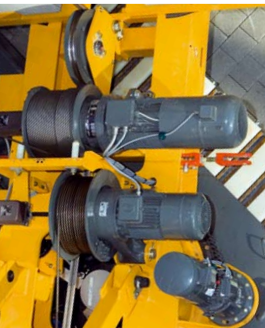
Hoisting and erecting winches.
